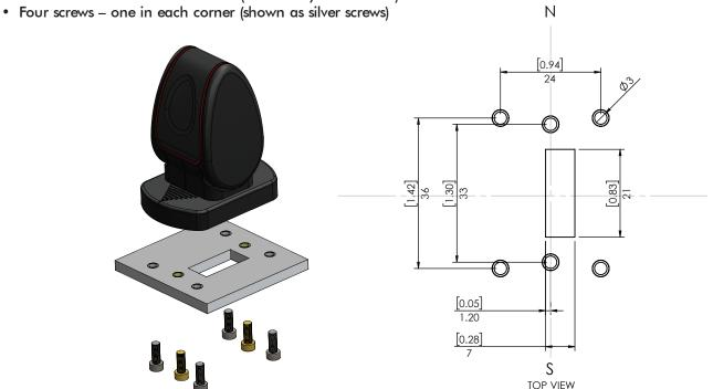
The Paddle is fitted with M3 bushes in all six positions, as standard.
