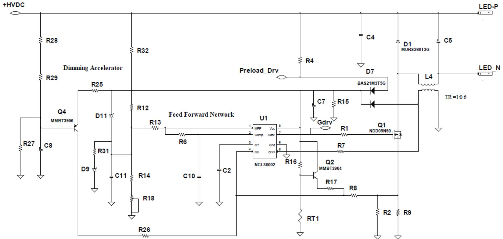
Figure 2 – Main Schematic
